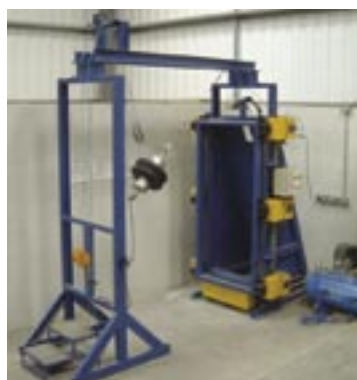
CGI's European Standards Impact Test Rig
