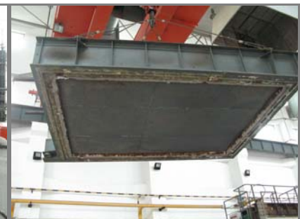
Lift off the furnace after a 4 hour fire test
